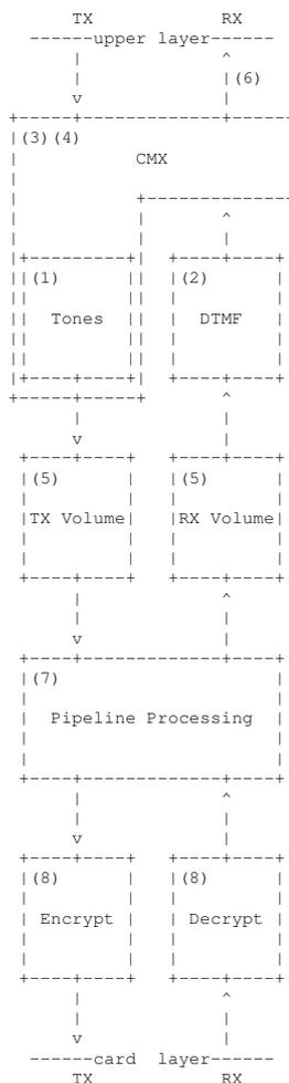
Data is ceiveived from card and decrypted, if crypto is enabled (8). Echo cancellation is performed (7), volume is changed (5) and DTMF digits are decoded (2). In bridfe mode, the data is relocked (3) (4) and forwarded to other member(s). Data is transmitted down from CMX (bridge). Tones are added, if enabled (1). The volume is changed (5), the echo cancellation is processed (7). The the data is encrypted, if enabled (8).
